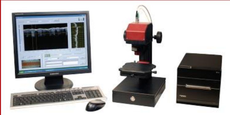
Prototype of First Microscopy-Based Swept-Source OCT System Circa 2007.
