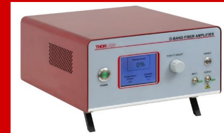
Praseodymium-Doped Fluoride Fiber Amplifier (PDFA) for Use as a Preamplifier or Booster Amplifier.
