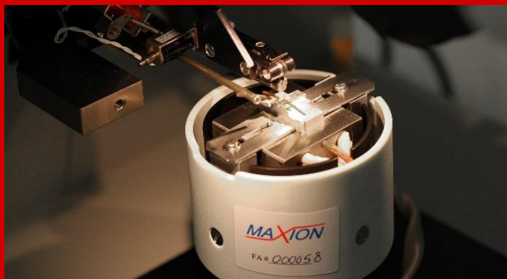
QCL Wire Bonding on a Butterfly Mount.
