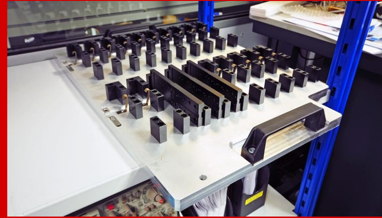
Testing Rig Uses T-Cube Controllers to Repeatedly Drive Actuators, Checking for Continual Use Faults.
