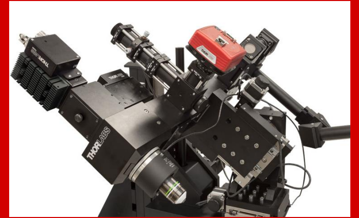
A Scientific CCD Camera Mounted to a Bergamo II Multiphoton Microscope.
